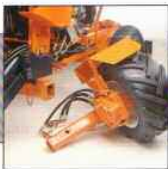
QUICK RELEASE FRONT AND REAR AXLES FOR DIFFICULT SITES
